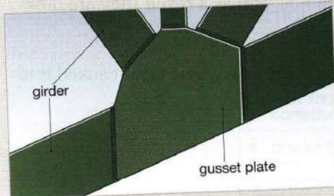
Fig. 1: Diagram showing the gusset plate joining two girders
